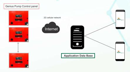
Supported protocol HTTP/HTTPS/FTP/MQTT/RAWTCP/IP
